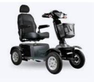
Excel Galaxy Roadmaster Plus Max weight capacity: 150kg Max speed: 8mph Max range\*: 35 miles
