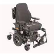
Otto Bock Juvo B6 MWD Tilt Max weight capacity: 140kg Max speed: 6mph Max range\*: 21 miles
